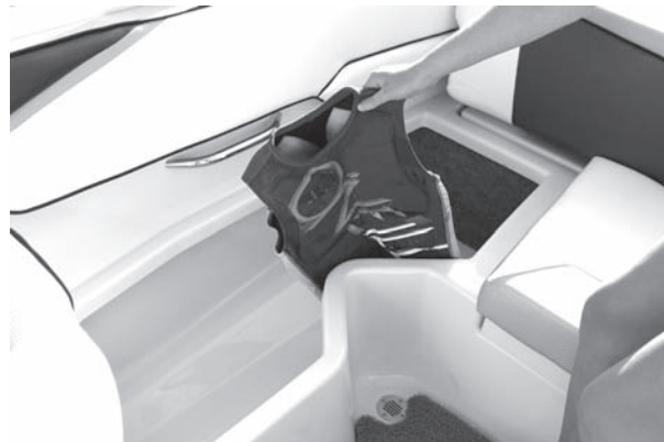
Figure C17: Starboard Cockpit Seat Cushion Storage
