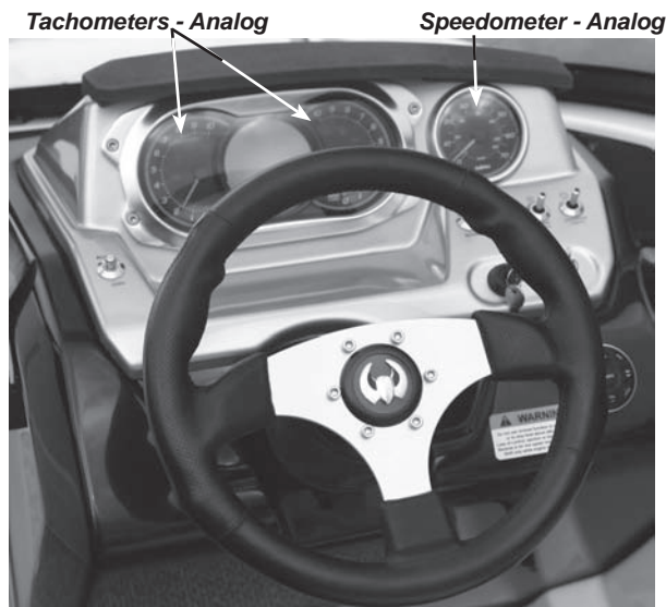
Figure B8: Information Center Gauges - Twin Engines
