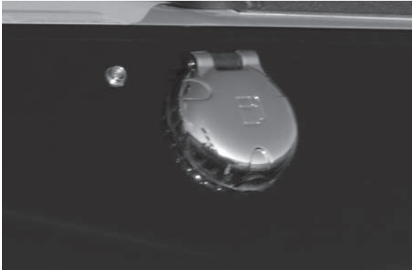
Figure B33: Fuel Deck Fill
