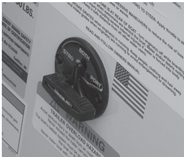
Figure B61: Port/Starboard Ballast Selector Switch
