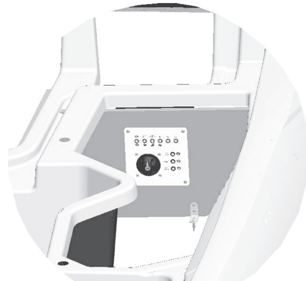
Figure B14: Battery Switch Panel Location (Location May Vary Depending on Model)
