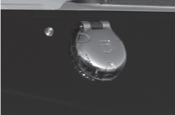
Figure B33: Fuel Deck Fill
