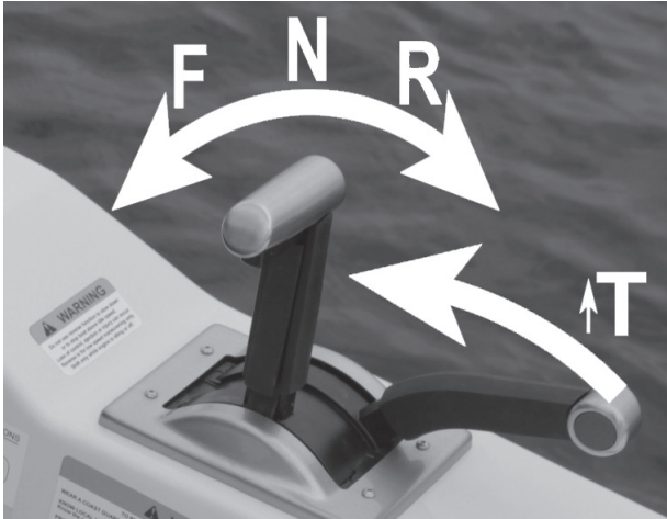
Figure D4: Separate Shift & Throttle Control Operation
