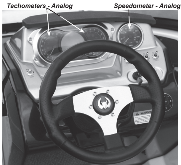
Figure B8: Information Center Gauges - Twin Engines
