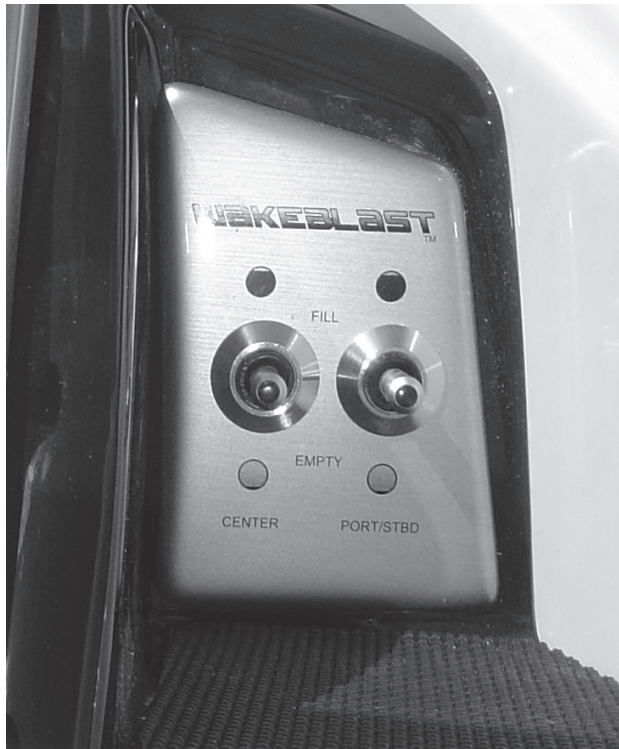
Figure B60: Ballast System Switch Panel
